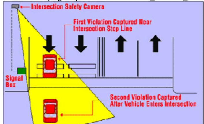
To detect speeding at intersections, these same sensors detect the presence of vehicles and calculate their speed using time and distance. If the speed of the vehicle exceeds the predetermined speed threshold, the camera will be triggered to photograph the violating vehicle as it passes through the intersection.
